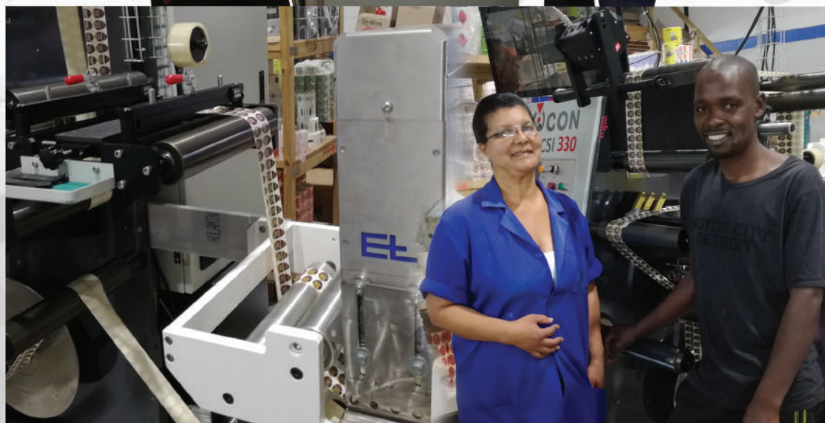
The RCSI 330 Ecoline is equipped with an Erhardt+Leimer (E+L) SmartScan inspection system – also supplied by Rotocon – a valuable tool for quality control in roll-label production. This finishing line is operated by Elizabeth Steenkamp and Topmore Mugudza.
