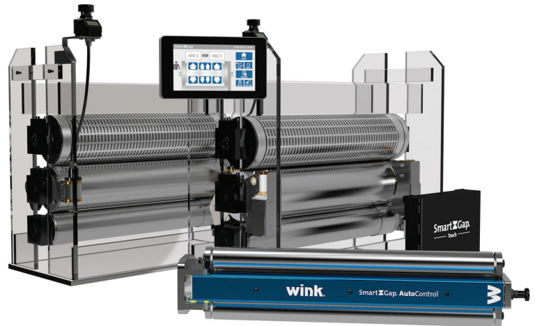
Wink's SmartGap AUTOCONTROL system has an adjustment range of 80µm and enables individual adjustment on the left and right and simultaneous adjustment on both sides in steps of 0.5µm down to 0.1µm.
