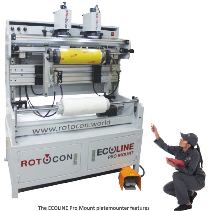
The ECOLINE Pro Mount platemounter features a 650-line camera that reaches 70 times amplification ratio and ensures clear, bright images on the high-resolution display screen.
