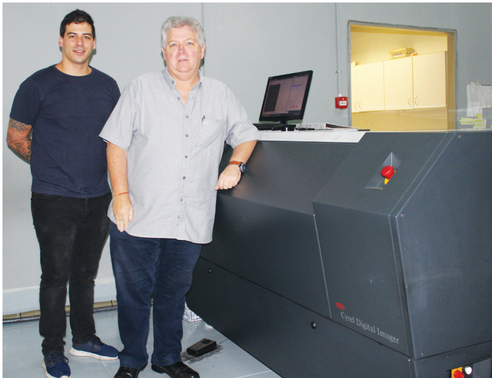
Stallion Repro's MD, Jeff Cutler (right), and platemaker, Storm Meyers, with the Esko CDI Spark 4835. It images all digital photopolymer plates, ranging from 0.76 to 6.35mm in thickness and up to 1 200 x 900mm in size.
